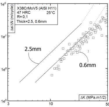
Figure 9. Comparison of Paris curves for thickness 2.5mm and 0.6mm at R=0.1
