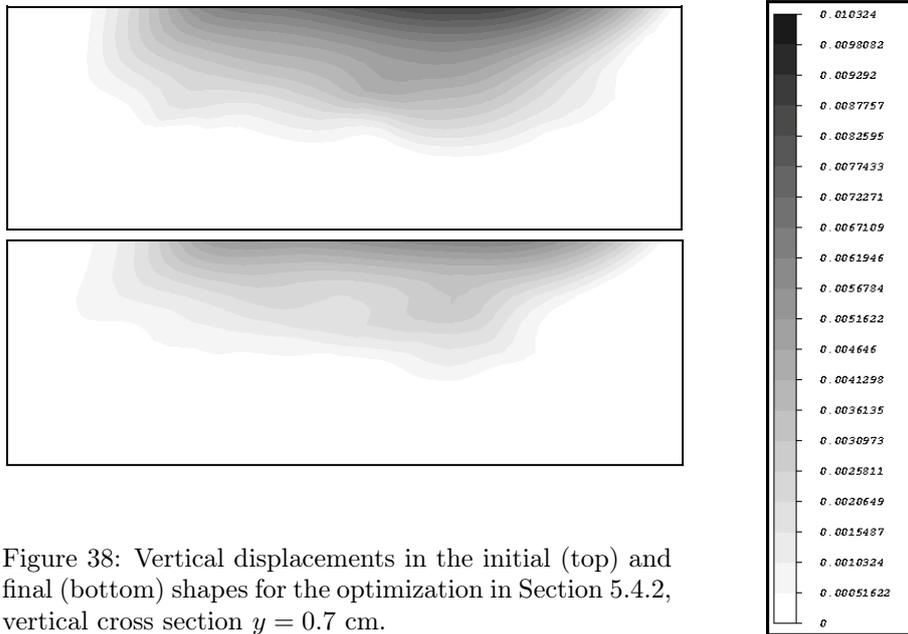
Figure 38: Vertical displacements in the initial (top) and final (bottom) shapes for the optimization in Section 5.4.2, vertical cross section  $y = 0.7$  cm.
