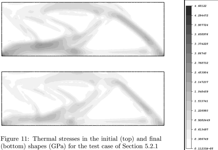
Figure 11: Thermal stresses in the initial (top) and final (bottom) shapes (GPa) for the test case of Section 5.2.1
