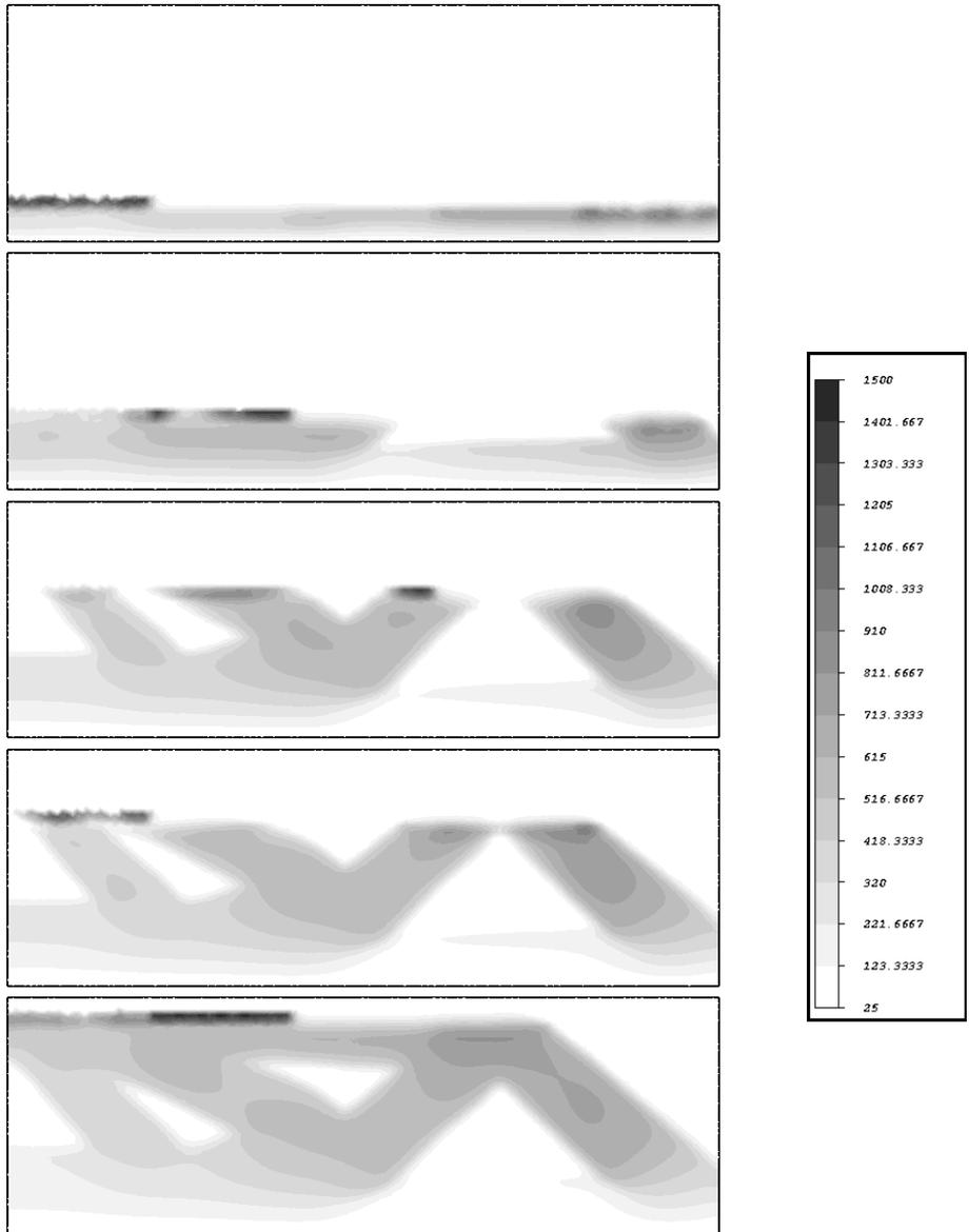
Figure 18: Temperature evolution during the building process for the layer by layer model of Section 3 at times  $t_3 + \Delta t, t_7 + 2\Delta t, t_{13} + 3\Delta t, t_{15} + \Delta t, t_{19} + 2\Delta t$ .
