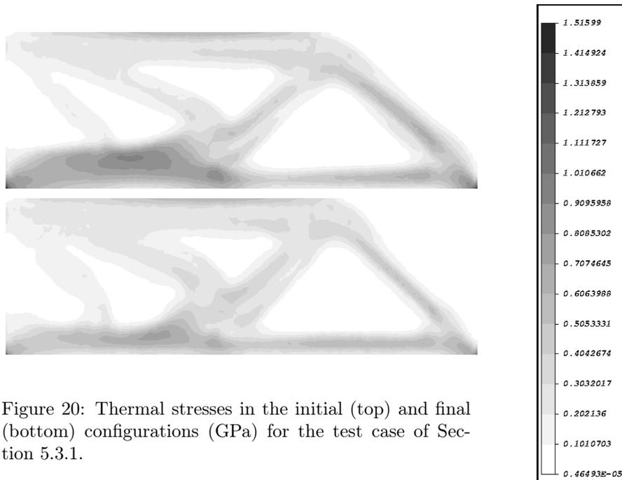
Figure 20: Thermal stresses in the initial (top) and final (bottom) configurations (GPa) for the test case of Section 5.3.1.
