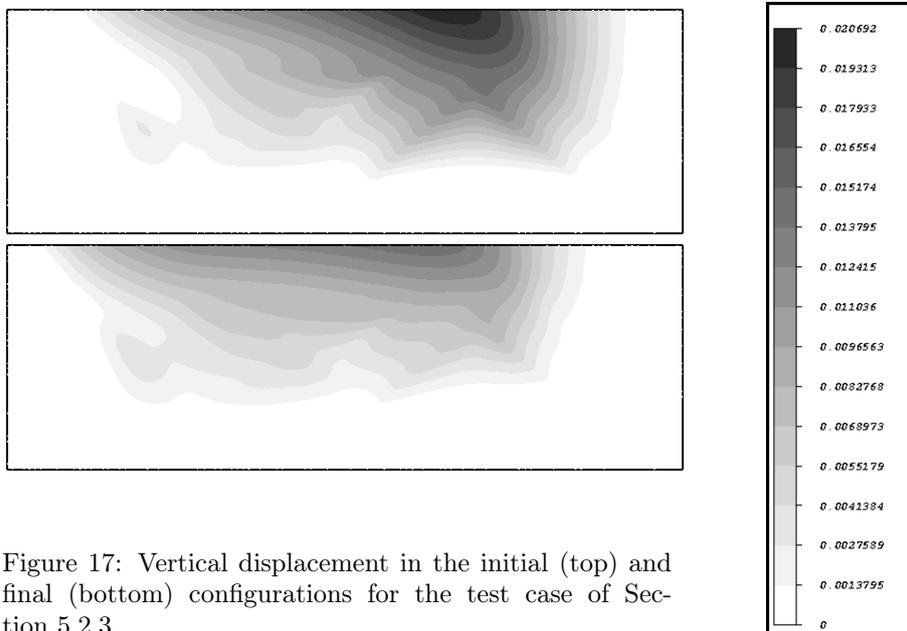
Figure 17: Vertical displacement in the initial (top) and final (bottom) configurations for the test case of Section 5.2.3
