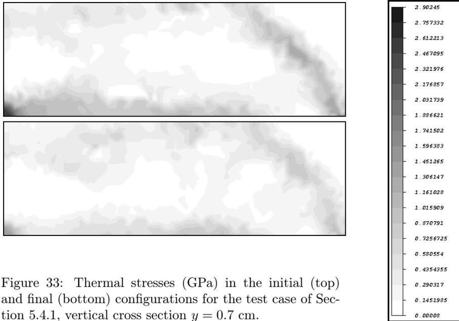
Figure 33: Thermal stresses (GPa) in the initial (top) and final (bottom) configurations for the test case of Section 5.4.1, vertical cross section  $y = 0.7$  cm.
