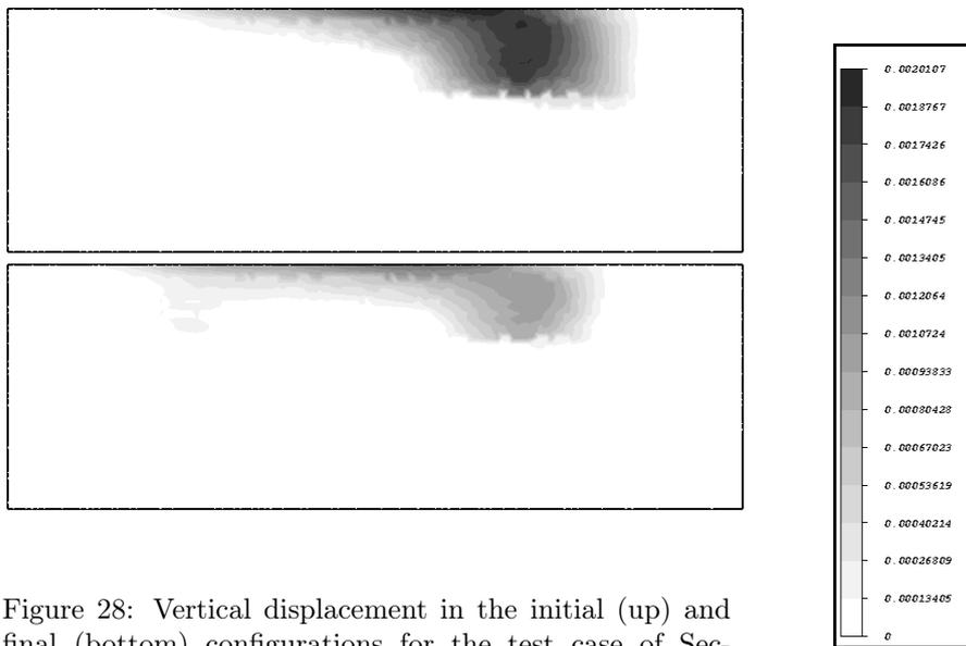
Figure 28: Vertical displacement in the initial (up) and final (bottom) configurations for the test case of Section 5.3.2.
