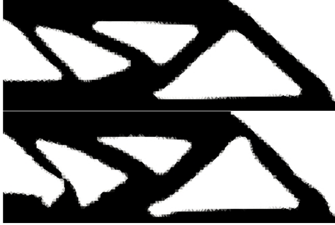
Figure 7: MBB beam initial (top) and final (bottom) shape for the test case of Section 5.2.1.
