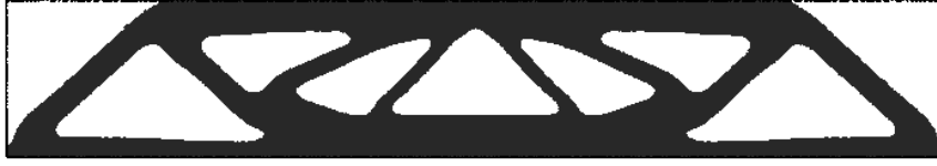
Figure 6: Optimal MBB beam for compliance minimization which is the initialization and reference shape for the constrained optimization (48)
