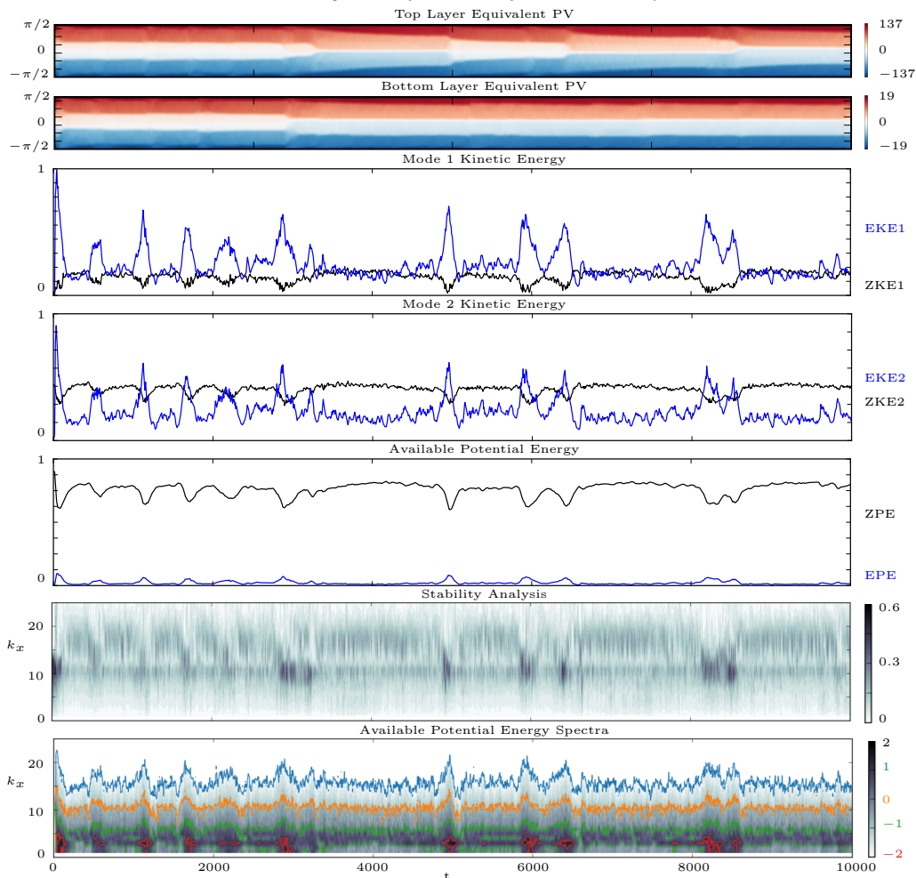
Figure 16: (a,b) Hövmoller diagrams of the equivalent PV, with latitude in the ordinate. (c,d,e) Energy components (with the eddy part in blue and the zonal part in black) versus time. (f) \log_{10} of the maximum growth rate of the zonally-averaged flow versus zonal wavenumbers. (g) \log_{10} of the y-integrated spectrum of the available potential energy versus zonal wavenumbers. For all these plots time is in the abscissa. The same parameters are used as in the characteristic simulation but on a 256 \times 128 basic inversion grid.
