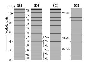
FIG. 2. Schematic view of the refined structure of *i*-Al-Pd-Mn projected normal to the fivefold axis (gray and black rectangles depict blocks of layers and gaps, respectively) showing (a) *medium* and *large gaps*, (b) only *large gaps*, (c) *large gaps* above regions of a moderate or high density, and (d) *large gaps* above regions of a high density.
