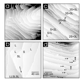
FIG. 1. STM images of the fivefold *i*-Al-Cu-Fe surface (a)–(d): (b) the area marked by white frame in image (a) in a magnified scale showing individual L and S steps, (c) steps formed with Fibonacci numbers of S and L steps, and (d) sequence of  $L(\rightarrow)$ ,  $S+L(\rightarrow)$  and  $S+2L(\Rightarrow)$  steps.
