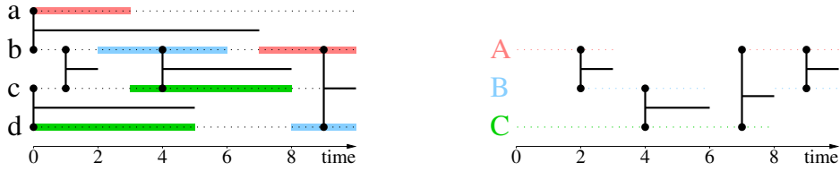
Figure 10: Example of quotient stream induced by a family of clusters. Left: a stream graph and a family F = (A, B, C) of clusters with A = [0, 3] \times \{a\} \cup [7, 10] \times \{b\} (in red), B = [2, 6] \times \{b\} \cup [8, 10] \times \{d\} (in blue), and C = [3, 8] \times \{c\} \cup [0, 5] \times \{d\} (in green). Right: the induced quotient stream. For instance, there is a link between A and C from time 7 to time 8 because there is a link between b and c at these times, and b is in A and c is on C at these times.
