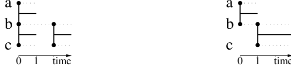
Figure 2: Two stream graphs with n = 2 nodes, m = 1 link, but with different densities: Left: \delta = 0.75 . Right: \delta = 1 .
