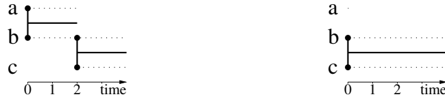
Figure 6: These two stream graphs have density 1 (all possible links exist), 2 nodes, and 1 link. However, the leftmost one has average node degree d(V) = \frac{|T_a|}{|W|}d(a) + \frac{|T_b|}{|W|}d(b) + \frac{|T_c|}{|W|}d(c) = \frac{2}{8}0.5 + \frac{4}{8}1 + \frac{2}{8}0.5 = 0.75 and the rightmost one has average node degree 1.
