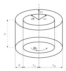
**Figure 1.** Taylor-Couette geometry.  $\mathbf{e}_r$ ,  $\mathbf{e}_\theta$  and  $\mathbf{e}_z$  are the unit vectors of the cylindrical coordinates system  $(r, \theta, z)$ .
