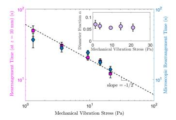
FIG. 8. Logarithmic plot of the rearrangement times  $\tau_R^*$  and  $\tau_{\rm vib}$  calculated with  $\langle \alpha \rangle$ , as functions of the mechanical vibration stress  $\sigma_v$ . The dashed line is a guide for the eyes. In the inset,  $\alpha$  vs  $\sigma_v$ .
