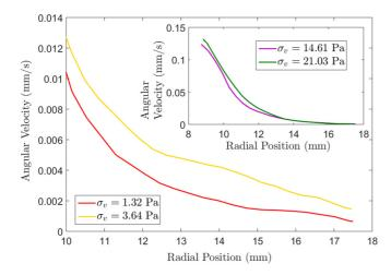
FIG. 6. Velocity profiles in the gap (at z=10 mm) for different values of mechanical vibration stress for an imposed shear stress  $\sigma=54$  Pa. In the inset,  $u_{\theta}$  vs r for some values of  $\sigma_{v}$  and for an imposed shear stress  $\sigma=70$  Pa.
