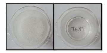
FIG. 2. Top view of the sample to test the readability of a text through 10 particle sizes. The sample is made of borosilicate beads of d=1 mm diameter in air (left), and the refractive index is matched with bidistilled glycerol (right): media and fluid have optical indexes equal  $n_D=1.473$ .
