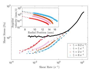
FIG. 5. Shear stress  $\sigma$  vs shear rate  $\dot{\gamma}$  for the case  $\sigma_v = 0$ . The solid line is data from the bulk rheology. Markers are data from the local rheology ( $\dot{\gamma}_{loc}$ ; $\sigma_{loc}$ ) obtained for various values of the imposed shear rates, well fitted to a fluidity model (dashed lines). In the inset, the logarithmic plot of the corresponding velocity profiles in the gap.
