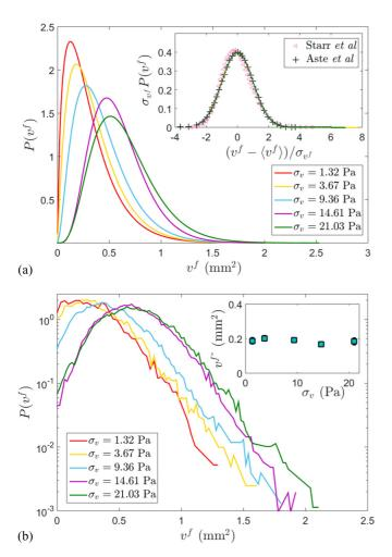
FIG. 9. Free volume distributions for different values of the mechanical vibration stress  $\sigma_v$ . (a) The data are well fitted with a  $\gamma$  law presented in Eq. (7) (solid lines). Inset: plot of the rescaled distributions. The same scaling has been found by Starr *et al.* [44] and Aste *et al.* [45]. (b) Semilogarithmic plot of raw data: well-defined exponential tails appear, with characteristic free volumes  $v^{f^*}$ . In the inset,  $v^{f^*}$  vs  $\sigma_v$ .
