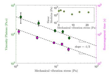
FIG. 4. Viscosity plateau  $\eta_0$  and rearrangement time  $\tau_R$  values, evaluated through Eq. (4), as functions of the mechanical vibration stress  $\sigma_v$ . In the inset, the shear modulus  $G_M$  vs  $\sigma_v$ . The dashed line is a guide for the eyes.
