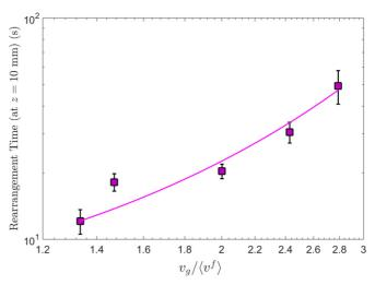
FIG. 10. Evolution of the rearrangement time  $\tau_R^*$  as a function of  $v_g/\langle v^f \rangle$ . The solid line is Doolittle's model presented in Eq. (8).
