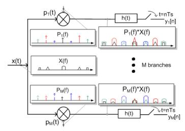
Fig. 1: Sensing process of the MWC.
