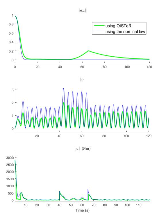
Figure 3.: Further comparison of the nominal and enhanced controllers through the tracking error  $(||q_{ev}(t)||)$ , the activity of the flexible modes  $(||\eta(t)||)$  and the control effort (||u(t)||).
