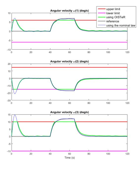
Figure 2.: Comparison of the angular velocities on each axis with the nominal and enhanced (OISTeR-based) control systems
