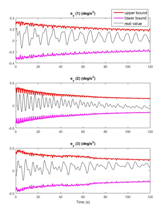
Figure 1.: Interval observer (bounds detection on the unmeasured disturbance torque  $e_y$ )
