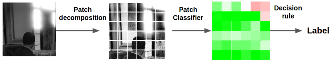
Fig. 1: Pipeline applied to a full-size image: patch decomposition, then patch classification, and finally results aggregation
