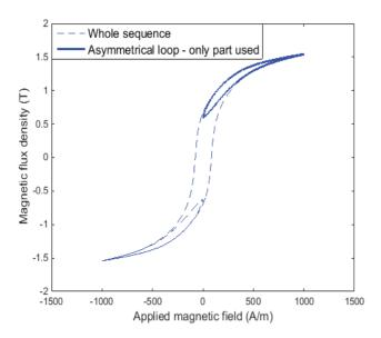
Fig. 3: Hysteresis loop with asymmetrical loop in NO20 - 1000A/m at 10Hz
