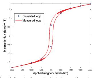
Figure 13: Comparison between simulated and measured hysteresis loop
