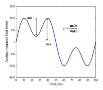
Fig. 5: Applied magnetic field waveform in NO20 - 1000A/m at  $10 \mathrm{Hz}$
