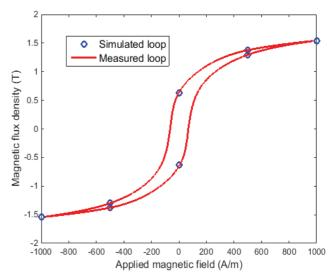
Fig. 9: Comparison between simulated and measured hysteresis loop for M = 2 in NO20 - 1000A/m at 10Hz
