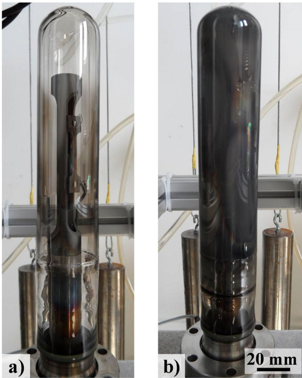
10 Illustration of sublimation after dwell at elevated temperature under secondary vacuum. (a) 1223 K – 14 h. (b) 1323 K – 6 h
