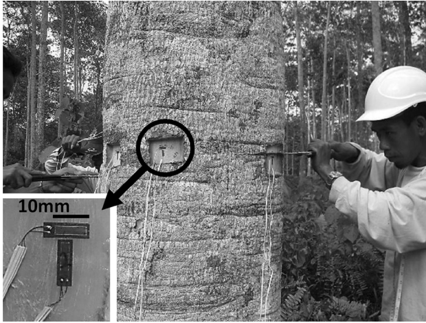
Fig. 6 Measurement of released strains of the surface growth stress using a 10 mm strain gauge (arrowheaded). At each measuring point, strain gauges are pasted parallel and perpendicular to the grain (Photo H. Yamamoto)
