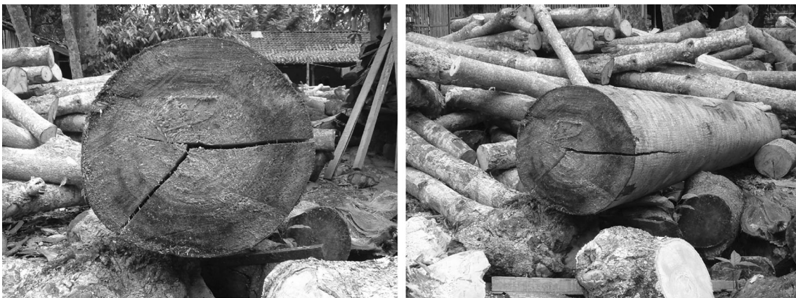
Fig. 17 Occurrence of radial cracks at the log end of Falcataria moluccana , harvested in Java Island, Indonesia (Photo H. Yamamoto)
