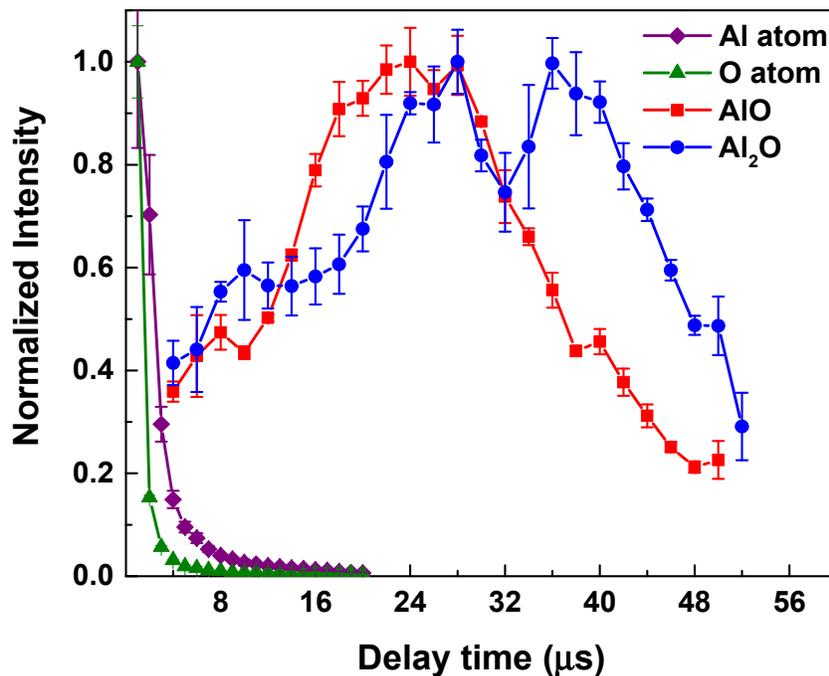
Fig. 4. Temporal evolution of the normalized emission intensities of Al I 308.2 nm (diamond dots), O I 777.2 nm (triangle dots), AlO 313.08 nm (square dots), and Al<sub>2</sub>O 261.40 nm (circle dots).
