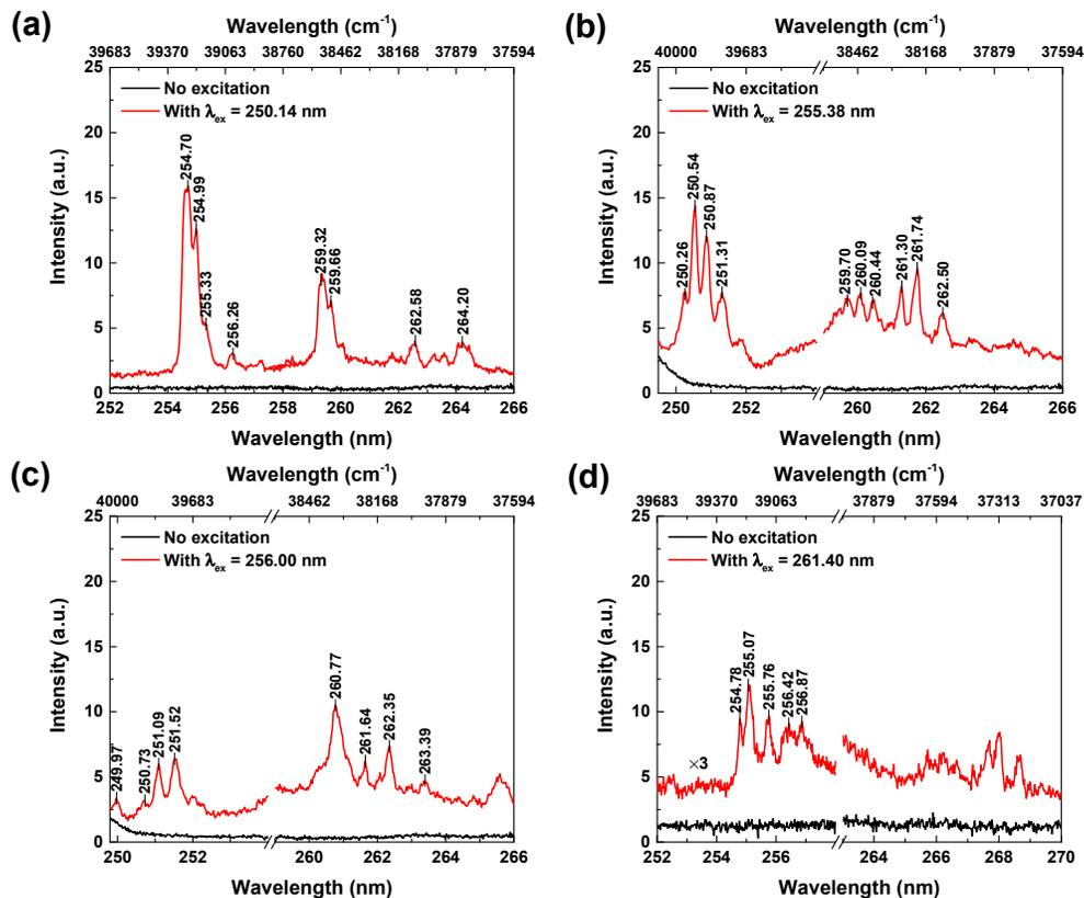
Fig. 3. Resonance fluorescence spectra of  $\text{Al}_2\text{O}$  with the excitation wavelengths at (a) 250.14, (b) 255.38, (c) 256.00, and (d) 261.40 nm measured with a gate width of 10 ns, an accumulation of 100 pulses, and a fixed interpulse delay time of 20  $\mu\text{s}$ .
