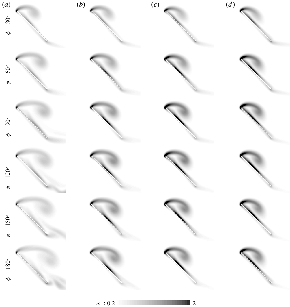
FIGURE 13. Contours of non-dimensional vorticity magnitude \omega^+ obtained in a spanwise cross-section located 2 chords away from the axis of rotation at 6 revolution angles (from top to bottom). Cases F_{co} = 0.5, 1, 1.5 and 2 (from a to d ) at Re = 500 and with F_{ce} = 1 .
