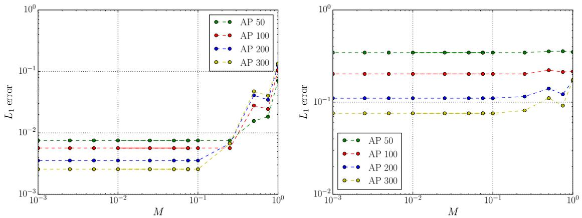
Figure 19: Density error (left) and velocity magnitude error (right) in terms of  $M$  for the AP scheme at time  $t = 1$  for different meshes (Taylor-Green vortex).
