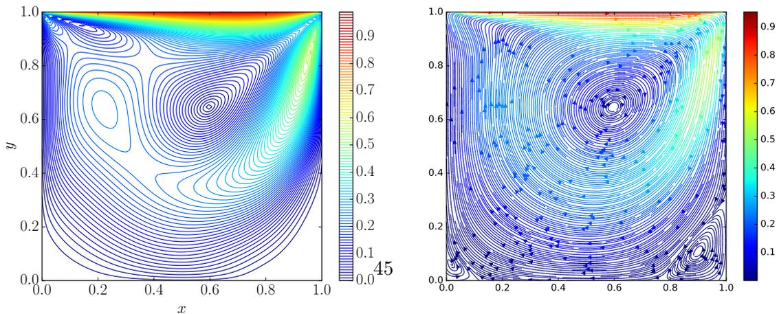
Figure 28: Contour plots of the velocity modulus (left) and velocity stream functions (right) for the AP scheme in the case  $\Delta x = \Delta y = 1/200$  for  $M = 0.2$  and  $Re = 400$  at time  $t = 30$ .
