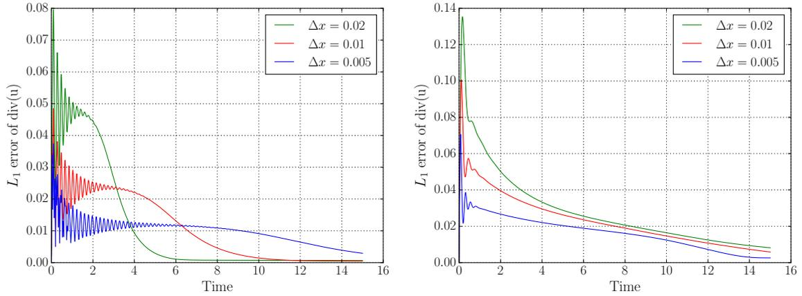
Figure 22: Temporal evolution of the  $L_1$  error of the velocity divergence for the relaxation scheme (left) and the AP scheme (right) in the case  $M = 0.1$  for different meshes (Taylor-Green vortex).
