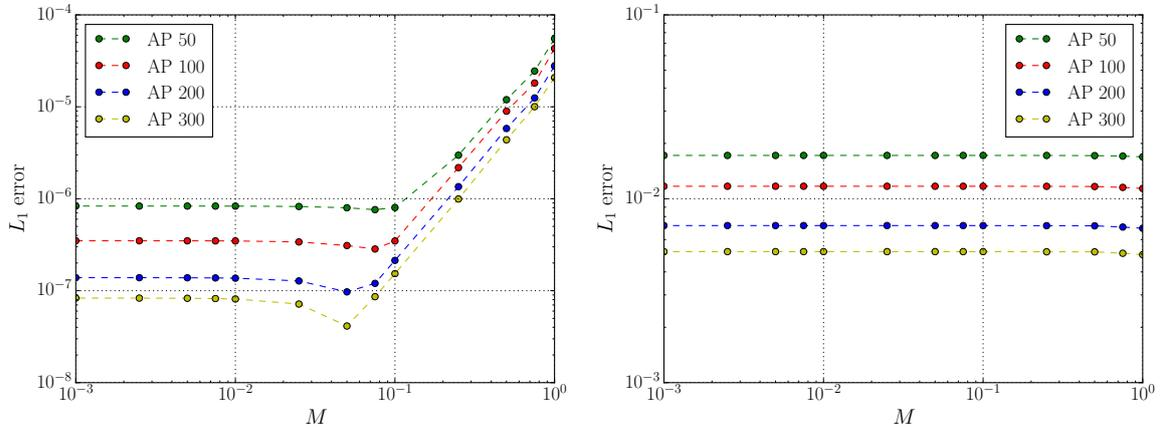
Figure 10: Density error (left) and velocity magnitude error (right) in terms of  $M$  for the AP scheme at time  $t = 0.1$  for different meshes (Travelling vortex).
