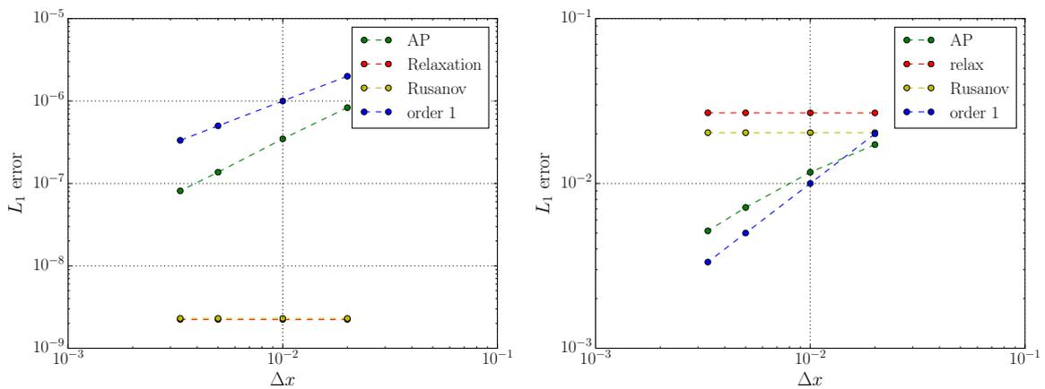
Figure 15: Density error (left) and velocity magnitude error (right) in terms of  $\Delta x$  for  $M = 0.01$  (Travelling vortex).
