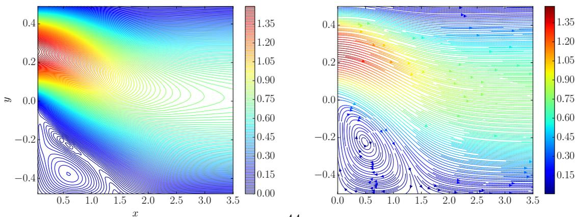
Figure 25: Contour plots of the velocity modulus (left) and velocity stream functions (right) for the AP scheme in the case  $\Delta x = 1/16$  and  $\Delta y = 1/32$  for  $M = 0.01$  and  $Re = 100$  at time  $t = 20$ .
