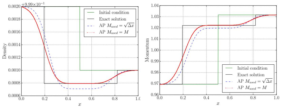
Figure 29: Limit of the approach: representation of the density (left) and momentum (right) at time  $t = 7 \times 10^{-3}$  in the case  $M^2 = 10^{-3}$  for  $M_{used} = \sqrt{\Delta x}$  (blue) and  $M_{used} = M$  (red).
