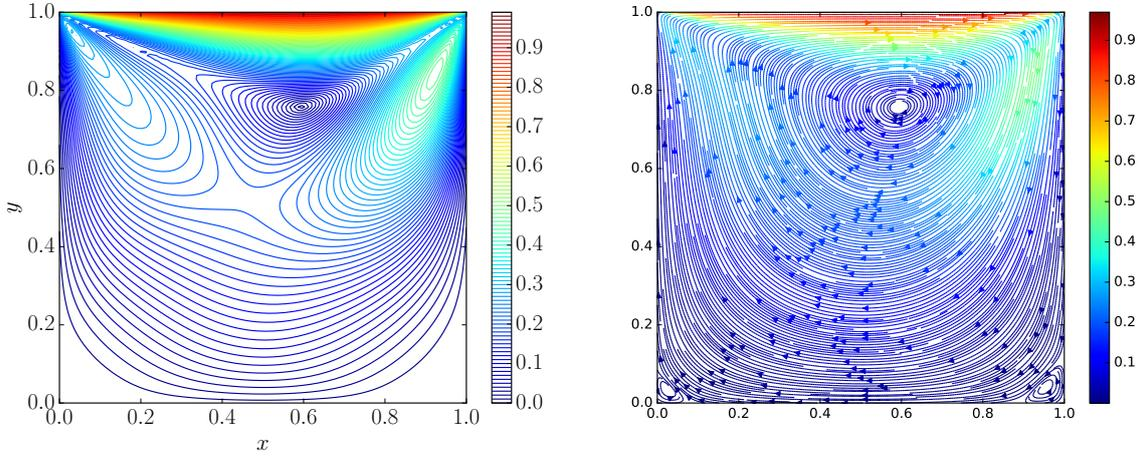
Figure 26: Contour plots of the velocity modulus (left) and velocity stream functions (right) for the Rusanov scheme in the case  $\Delta x = \Delta y = 1/200$  for  $M = 0.2$  and  $Re = 400$  at time  $t = 30$ .
