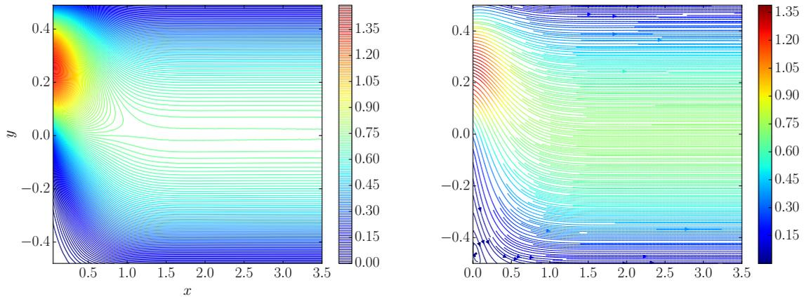
Figure 23: Contour plots of the velocity modulus (left) and velocity stream functions (right) for the Rusanov scheme in the case  $\Delta x = 1/16$  and  $\Delta y = 1/32$  for  $M = 0.01$  and  $Re = 100$  at time  $t = 20$ .
