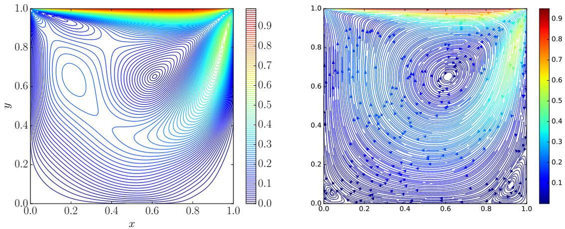
Figure 27: Contour plots of the velocity modulus (left) and velocity stream functions (right) for the relaxation scheme in the case  $\Delta x = \Delta y = 1/200$  for  $M = 0.2$  and  $Re = 400$  at time  $t = 30$ .
