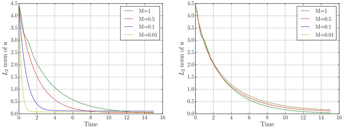
Figure 21: Temporal evolution of the  $L_2$  norm of the velocity for the relaxation scheme (left) and the AP scheme (right) in the case  $50 \times 50$  for different  $M$  (Taylor-Green vortex).
