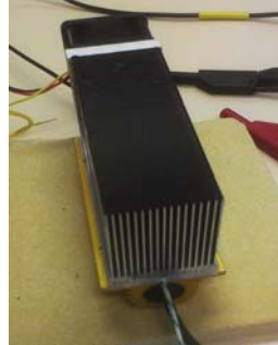
Fig. 6. Manufactured heat sink used to verify the accuracy on thermal resistance model having 10 elements in the resistance network. Weight = 0.286kg and thermal resistance = 0.23K/W.
