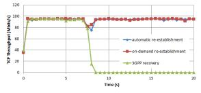
Fig. 7: TCP throughput under SGW failure.
