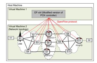
Fig. 6: Test topology in Mininet.
