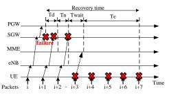
Fig. 5: Timing diagram of 3GPP recovery mechanism.
