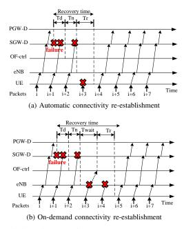
Fig. 4: Timing diagram of SDN-based recovery mechanisms.
