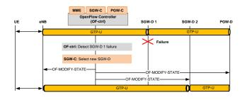
Fig. 2: Automatic connectivity re-establishment. Here, we can see the advantage of logical centralizing the TEID allocation function related to SGWs. Indeed, the SGW-C does not create new TEID values during the recovery mechanism. The OF-ctrl updates just flow entries in eNB and PGW-D with the new SGW-D IP address. However, the OFctrl inserts a new flow entry in SGW-D 2 to enable traffic forwarding between eNB and PGW-D.
