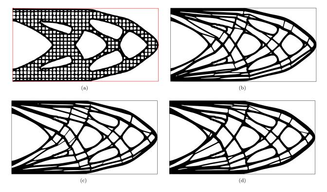
FIGURE 29. (a) initial infill design  $\omega^0$  for the second stage of the two-step process for non regular infill design in the cantilever example of Section 8.3.1; (b-d) optimized shapes  $\omega$  having the same compliance as  $\omega^0$  setting (b)  $\delta = 3\Delta x$ , (c)  $\delta = 4\Delta x$  and (d)  $\delta = 5\Delta x$ .
