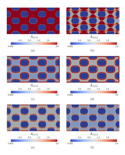
FIGURE 11. Distribution of the elastic coefficient  $A_{1111}$  using the six considered models for the elastic properties of shapes in the cantilever test case of Section 8.2.1.
