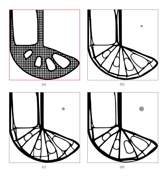
FIGURE 31. (a) initial infill design  $\omega^0$  for the second stage of the two-step process for non regular infill design in the L-beam example of Section 8.3.2; (b-d) optimized shapes  $\omega$  having the same compliance as  $\omega^0$  setting (b)  $\delta = 4\Delta x$ , (c)  $\delta = 5\Delta x$  and (d)  $\delta = 8\Delta x$ .
