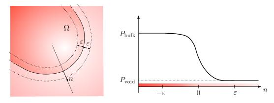
FIGURE 7. Interpolation of any of the (scalar) entries P of the Hooke's tensor  $A_{\Omega}^{\text{off}}$  using the 'offset' model (5.10).
