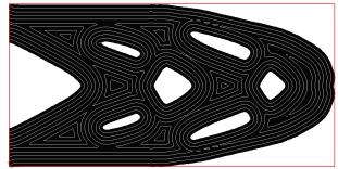
FIGURE 13. Optimized shapes  $\Omega^*$  and  $\Omega$  for the two-dimensional cantilever test case of Section 8.2.1 in (left) the 'molded' case (a), and (right) the 'offset' model (b).
