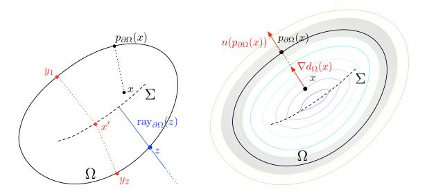
FIGURE 5. (Left) Projection point  $p_{\partial\Omega}(x)$  of  $x \in \Omega$ , projection set  $\Pi_{\partial\Omega}(x') = \{y_1, y_2\}$  of another point  $x' \in \Omega$  and ray emerging from  $z \in \partial\Omega$ ; (right) the gradient of  $d_{\Omega}(x)$ , if it is defined, equals the normal vector to  $\partial\Omega$  at  $p_{\partial\Omega}(x)$ .
