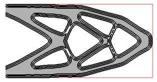
(f) 'Crust-pattern model' with anisotropic crust and isotropic infill
