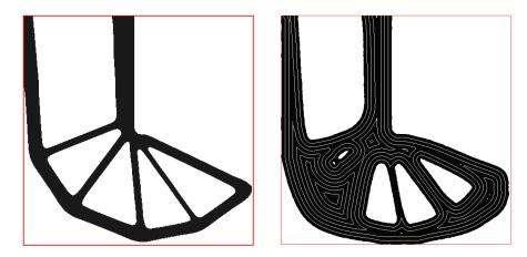
FIGURE 19. Optimized shapes  $\Omega^*$  and  $\Omega$  obtained in the L-shaped beam test case of Section 8.2.2 (left) in the 'molded' situation, (right) when the material properties of shapes are described using the 'offset' model.
