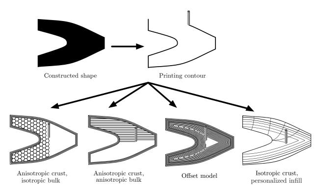
FIGURE 2. Construction of one 2d layer of a 3d structure with the FFF technology. (Top-left) outline of the layer; (top-right) construction of the contour; (bottom, from the left to the right) assembly of the bulk of the layer using an isotropic infill, an anisotropic (horizontally oriented) infill, along contour offsets, and using a personalized infill.
