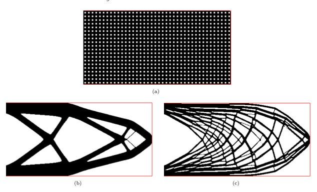
FIGURE 27. (a) Initial design, and (b) optimized two-dimensional cantilever obtained in Section 8.3.1 without imposing any thickness constraint (i.e. (8.2) is solved); (c) optimized two-dimensional cantilever for (8.4) with  $\delta = 10\Delta x$ .
