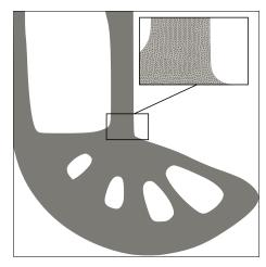
FIGURE 30. First step of the two-step process for non regular infill design in the L-beam example of Section 8.3.2; (left) optimized shape considering shapes with an isotropic crust and an isotropic infill with density 0.6; (Right) exported unstructured mesh, used as a new design domain for the second step.
