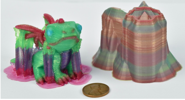
Fig. 14. 3D printed dragon with its supports and its priming shield.
