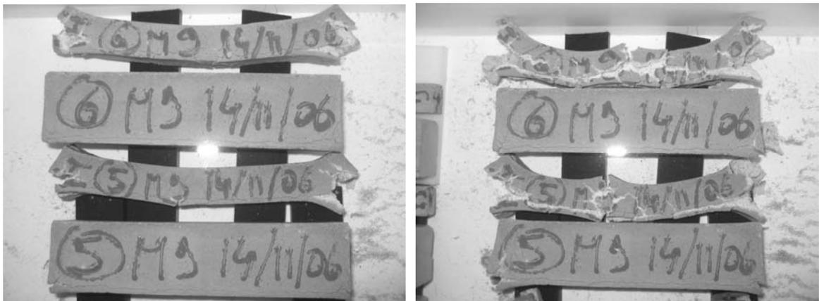
Figure 1 : Degradation of mortars samples ( $4*4*16$  cm<sup>3</sup> and  $2*2*16$  cm<sup>3</sup>) submitted to sulphate attacks at 135 days and 150 days [4].
