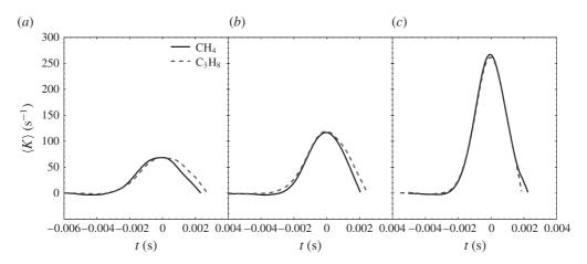
FIGURE 6. Time evolution of the stretch rate for stoichiometric methane and lean  $(\phi = 0.9)$  propane/air mixtures for three different vortex strengths and  $\Delta = 13$  mm: (a)  $U_{\theta}/\langle S_c^1 \rangle_{t_0} = 0.8$ , (b)  $U_{\theta}/\langle S_c^1 \rangle_{t_0} = 1.2$ , (c)  $U_{\theta}/\langle S_c^1 \rangle_{t_0} = 2.8$ . The time t has been shifted so that t = 0 corresponds to the time at which  $\langle K \rangle$  is maximum.
