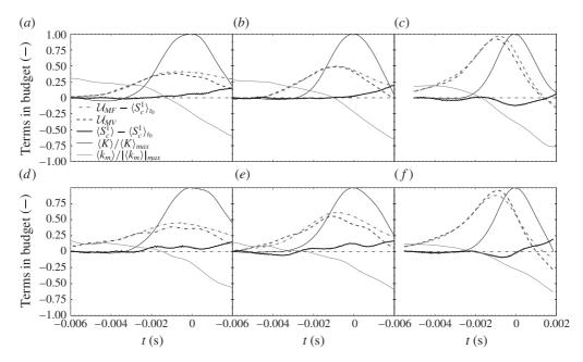
FIGURE 11. Time evolution of the different terms in (3.22) normalized by  $\langle S_c^1 \rangle_{t_0}$ . The vortex intensity  $U_\theta / \langle S_c^1 \rangle_{t_0} = 0.8$  (a,d), 1.2 (b,e) and 2.8 (c,f). Stoichiometric CH<sub>4</sub>/Air mixture (a-c), lean ( $\phi = 0.9$ ) C<sub>3</sub>H<sub>8</sub>/Air mixture (d-f).
