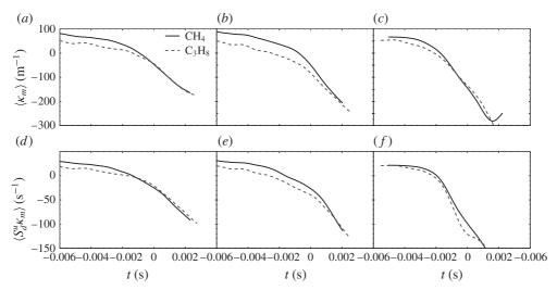
FIGURE 7. Time evolution of  $\langle \kappa_m \rangle$  (a-c) and  $\langle S_d^u \kappa_m \rangle$  (d-f) for stoichiometric methane and lean  $(\phi=0.9)$  propane/air mixtures for three different vortex strengths: (a,d)  $U_\theta/\langle S_c^1 \rangle_{t_0} = 0.8$ , (b,e)  $U_\theta/\langle S_c^1 \rangle_{t_0} = 1.2$ , (c,f)  $U_\theta/\langle S_c^1 \rangle_{t_0} = 2.8$ . The time t has been shifted so that t=0 corresponds to the time at which  $\langle K \rangle$  is maximum.
