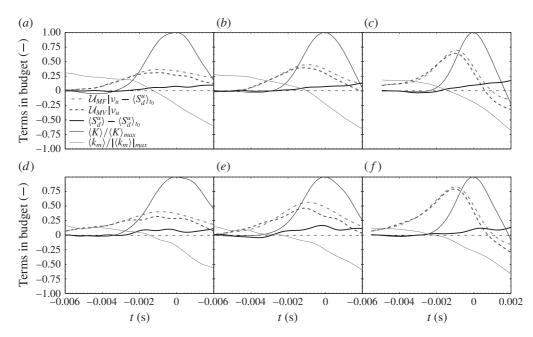
FIGURE 8. Time evolution of the different terms in (3.11), normalized by  $\langle S_d^u \rangle_{t_0}$ . The vortex intensity  $U_\theta/\langle S_c^1 \rangle_{t_0} = 0.8$  (a,d), 1.2 (b,e) and 2.8 (c,e). Stoichiometric CH<sub>4</sub>/Air mixture (a-c), lean ( $\phi = 0.9$ ) C<sub>3</sub>H<sub>8</sub>/Air mixture (d-f). The time t is translated so that t = 0 corresponds to the maximum of total stretch rate.
