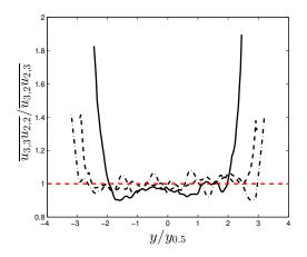
FIG. 10. Distributions across the wake of  $\overline{u_{2,2}u_{3,3}}/\overline{u_{2,3}u_{3,2}}$  involved in Eq. (8) at x = 20D (solid line), 60D (dashed line) and 100D (dot-dashed line). Red dashed line: Isotropic value of 1.
