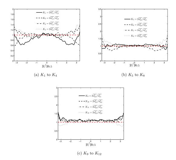
FIG. 9. Distributions across the wake of ratios  $K_1$  to  $K_{12}$  at x/D = 100, (a)  $K_l$  to  $K_4$ ; (b)  $K_5$  to  $K_9$ ; (c)  $K_9$  to  $K_{12}$ . Red dashed line, Isotropic value of one.
