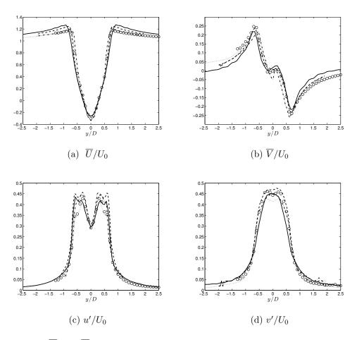
FIG. 5. Profiles of  $\overline{U}$  (a),  $\overline{V}$  (b), u' (c) and v' (d) at x/D = 0.54. Solid line: LBM; doted line: PIV-2C<sup>33</sup>; dashed-dotted line: DNS<sup>27</sup>; dashed line: LES<sup>21</sup>; symbols: ADL3C measurements<sup>33</sup>.
