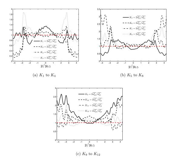
FIG. 7. Distributions across the wake of ratios  $K_1$  to  $K_{12}$  at x/D = 20, (a)  $K_l$  to  $K_4$ , ; (b)  $K_5$  to  $K_9$ ; (c)  $K_9$  to  $K_{12}$ . Red dashed, Isotropic value of 1.
