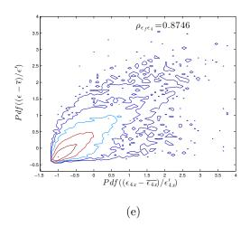
FIG. 13. Joint probability density function of the turbulent kinetic energy dissipation (Eq. (1) and Eq. (2), (5), (6), (3), (9) at position y = 0 and x/D = 100.
