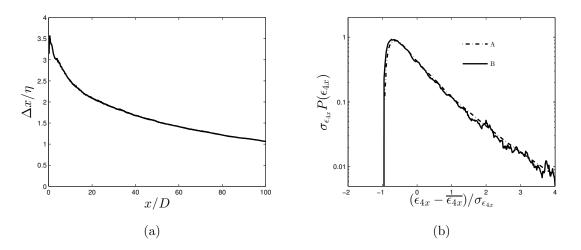
FIG. 2. (a) Variation of  $\Delta x/\eta$  with x along the axis of the SqC wake. (b) Probability density function of the turbulent kinetic energy dissipation inferred from Eq. (9) at x/D = 100 on the centerline. Solid line: present data (SC) ; dashed dotted line: DNS from Antonia et al.<sup>3</sup> using Eq. (9).
