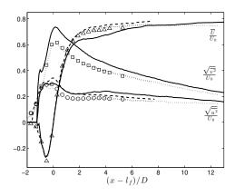
FIG. 4. Streamwise distributions of  $\overline{U}/U_0$ ,  $u'/U_0$  and  $v'/U_0$ , on the centerline of a CC wake. Solid line: LBM; dashed line: LES ; dotted line: PIV-2C<sup>33</sup>; symbols: ADL3C<sup>33</sup> measurements.
