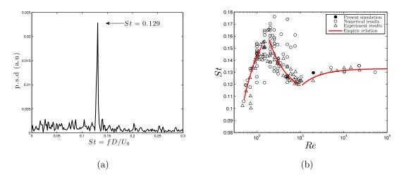
FIG. 3. (a) Spectra of  $\epsilon$  at x/D = 20 and y/D = 4. (b) Variation of the Strouhal number with the Reynolds number. Experimental results<sup>12,23,26,28</sup>; Numerinal results<sup>24,28</sup>
