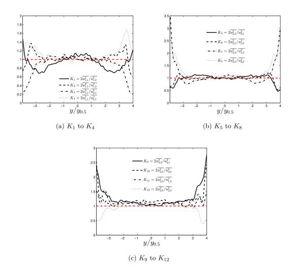
FIG. 8. Distributions across the wake of ratios  $K_1$  to  $K_{12}$  at x/D = 60, (a)  $K_l$  to  $K_4$ , ; (b)  $K_5$  to  $K_9$ ; (c)  $K_9$  to  $K_{12}$ . Red dashed line, Isotropic value of 1.
