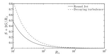
FIGURE 1.  $S + 2G/R_{\lambda}$  as a function of  $R_{\lambda}$  in decaying (dashed line) and on the axis of a round jet (solid line). For the purely decaying flow,  $\mathcal{R} = 1$  and  $n_u = 1$  whereas for the jet flow  $\mathcal{R} = 2/3$ .
