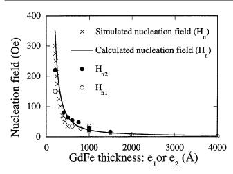
FIG. 4. Measured  $[H_{n1}(e_1)]$  and  $H_{n2}(e_2)$ , calculated and simulated nucleation fields plotted as a function of the GdFe thicknesses  $e_1$  or  $e_2$ . The nucleation fields were calculated from relation (4).
