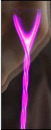
Fig. 8. Discharge observed at low pressure in a twisted pair of enamel wires fed by Pulse like voltage.
