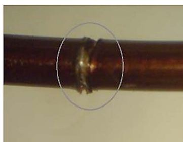
Fig. 5: View of a ring defect on the enameled wire
