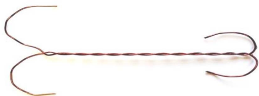
Fig. 1: Standard twisted pair of low-voltage winding
