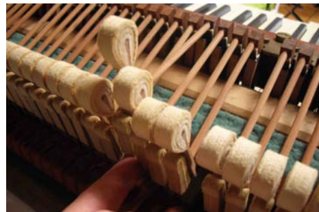
Figure 1: New hammers of the Pleyel piano E.991.16.1 from 1842 (collection of the Paris Museum of Music). Facsimile made in 2014 by the French piano maker Maurice Rousteau.
