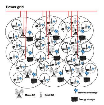
Fig. 1. Nework of macro BSs powered by RE and the power grid overlapped by small BSs powerd by RE.
