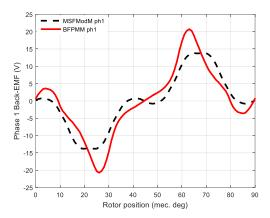
Fig. 14. Open-circuit phase back-EMF waveforms
