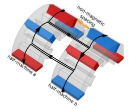
Fig. 8. Axial flux path
