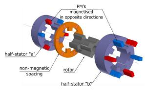
Fig. 2. MSFModM 3D exploded view
