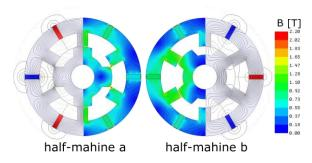
Fig. 4. Open-circuit induction distribution and flux lines at rotor position  $\theta = 0^{\circ}$
