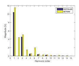
Fig. 15. Open-circuit phase back-EMF spectrum
