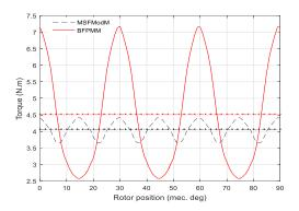
Fig. 16. Torque vs rotor position ( $I_{RMS}$ = 7.7 A)
