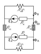
Fig. 9. MEC model for 3-D leakage flux correction
