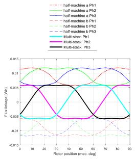
Fig. 5. Open-circuit flux linkage
