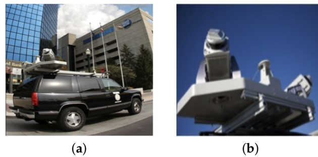
Figure 1. (a) The Vis Center’s LiDAR Truck. (b) Two Optech LiDAR sensor heads, a GPS, an inertial measurement unit and a spherical digital camera mounted on a rigid frame.
