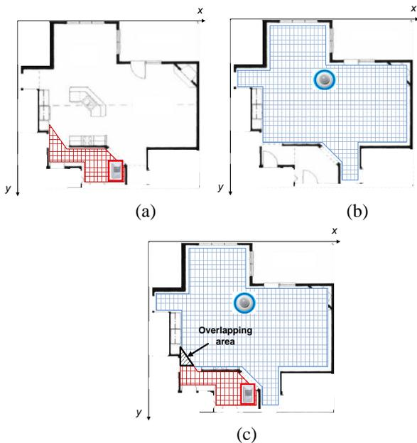
Fig. 7. The first solution of set  $\mathcal{S}(a)$ : (a) sensor of type 1; (b) sensor of type 7; (c) overlapping area of the two sensors.
