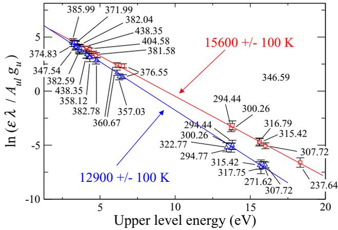
FIG. 2. Saha-Boltzmann plot of Fe and Fe<sup>+</sup> transitions for  $t = 230$  ns (squares) and 500 ns (triangles).
