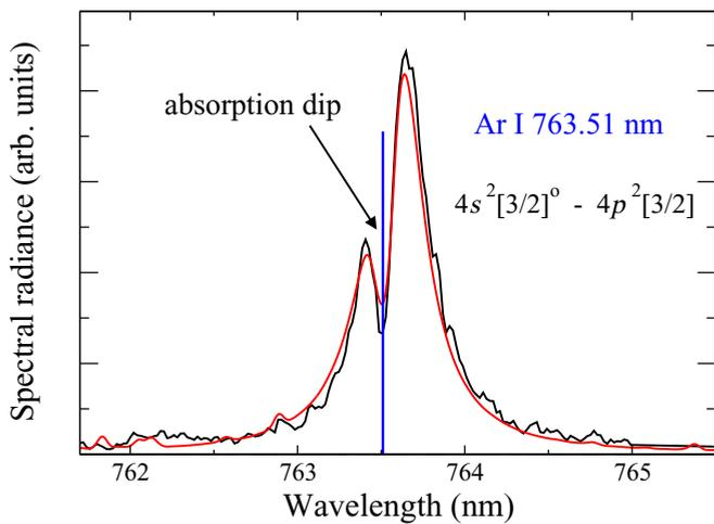
FIG. 5. Measured (black line) and computed (red line) shapes of an Ar transition toward the metastable state. The recording was performed during ablation of steel for  $t = 500$  ns. The simulation was obtained by adding two layers to the laser plasma, representing the heated gas at the vapor-gas contact front and the adjacent colder gas. The absorption dip was observed for each investigated material.
