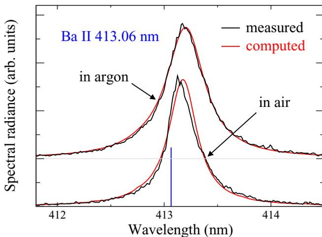
FIG. 3. Ba II 413.06 nm line profile recorded during laser ablation of barite crown glass for  $t = 500$  ns. Comparison to the spectral radiance computed for a uniform LTE plasma. The blue line indicates the resonance wavelength of the transition.
