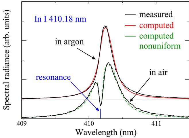
FIG. 4. In I 410.18 nm resonance line recorded during laser ablation of indium for  $t = 500$  ns. The measurements in argon and air are compared to the spectral radiances of a uniform and a nonuniform LTE plasma, respectively.
