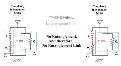
**Figure A.6.2.** After quantum measurement the entanglement link is disrupted, however, this persists in a ghostly way. Both resulting spins will be completely independent, and the action of the decoherence is represented with resistors in inductors and capacitors.
