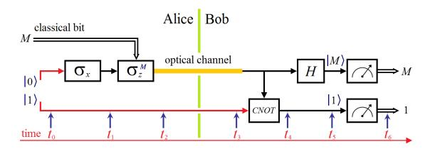
**Figure A.7.6.** Proposed SDC protocol with only one classical bit to be transmitted using a  $(|0\rangle, |1\rangle)$  pair.
