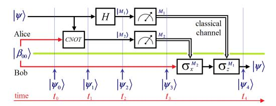
Figure A.7.1. Standard Teleportation protocol using an EPR pair and two classical bits for disambiguation.
