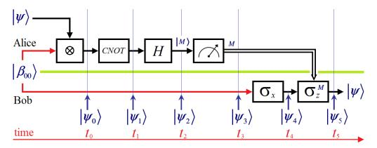
**Figure A.7.2.** Proposed Teleportation protocol with only one classical bit of disambiguation and using an EPR pair.
