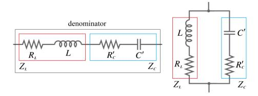
Figure A.2.6. RLC circuit of Fig.A.2.5 with a built-in simplification on the original RC circuit.
