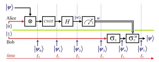
**Figure A.7.3.** Proposed Teleportation protocol with only one classical bit of disambiguation and using a  $(|0\rangle, |1\rangle)$  pair.
