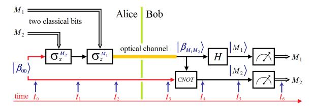
Figure A.7.4. Standard SDC protocol with two classical bits to be transmitted and using an EPR pair.
