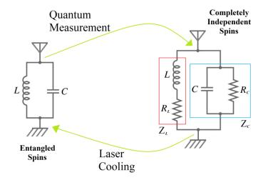
**Figure A.6.4.** For a given EPR element, the upper green arrow shows the pass from the entangled spins to completely independent spins via quantum measurement, while, the bottom green arrow indicates the transition from completely independent spins to entangled spins thanks to laser cooling. Laser cooling eliminates the resistors factors that inhibit the entanglement.
