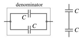
Figure A.2.3. A capacitive version of completely independent subsystems.
