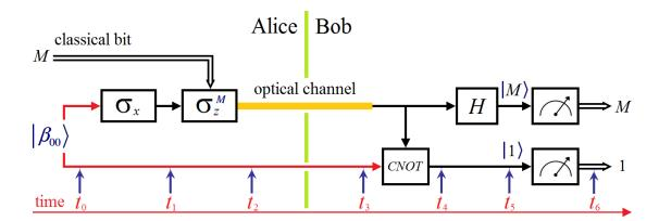
Figure A.7.5. Proposed SDC protocol with only one classical bit to be transmitted using a EPR pair.
