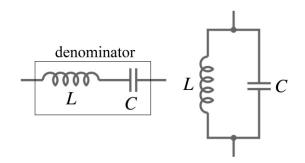
Figure A.2.1. On the left we have a serial LC circuit which is the denominator of Eq.(A.2.5), and on the right we have a parallel LC circuit.
