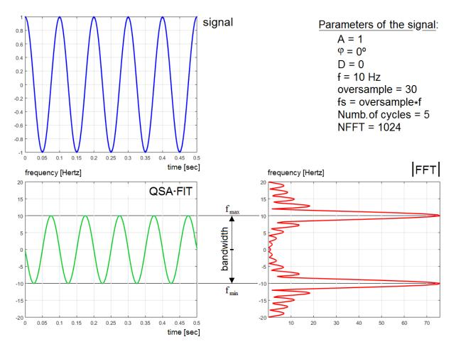
Fig. 18 Example of signal (in blue), QSA-FIT (in green), and |FFT| (in red) of cosine.
