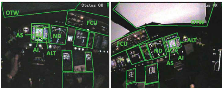
Figure 1. An example of reference images and areas of interests (AOIs) for pilot flying (at left) and pilot monitoring (at right). We focused our analyses on the six AOIs that received the majority of scans: airspeed (AS), attitude indicator (AI), altitude indicator (ALT), navigation display (ND), flight control panel (flight control unit for Airbus and mode control panel for Boeing), and out of the window (OTW).
