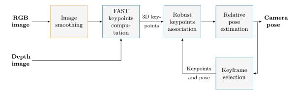
Figure 3: The pipeline of the Fovis algorithm. The preprocessing and registration steps are displayed in orange and blue respectively.
