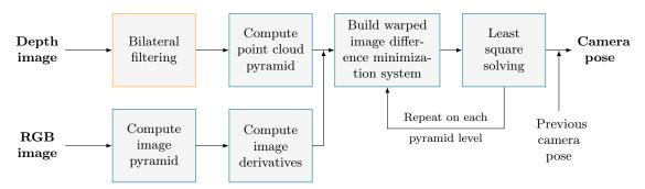
Figure 4: The pipeline of the OCV RGB-D algorithm.
