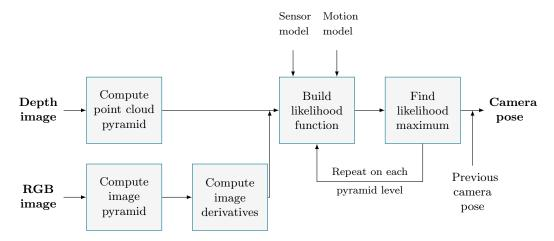
Figure 7: The pipeline of the DVO algorithm.
