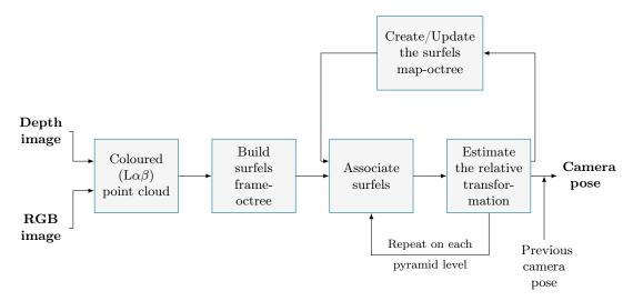
Figure 8: The pipeline of the MRSMap algorithm. The nodes association and transformation estimation steps are parallelized for each node and association respectively.
