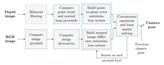
Figure 6: The pipeline of the OCV RgbdICP algorithm.
