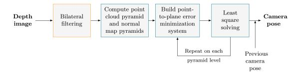
Figure 5: The pipeline of the OCV ICP algorithm.
