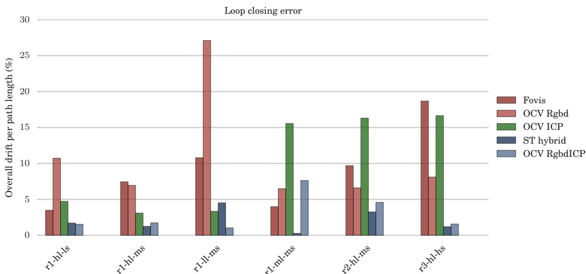
Figure 13: Loop closing error defined as the distance between the endpoints of the estimated trajectory divided by the path length.
