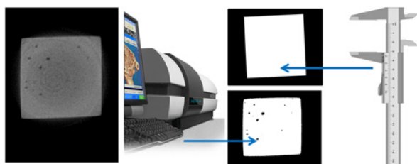
Fig. 2. \mu CT-scan measurement – (a) Bone area cross section of the sample, (b) Comparison between classical cross section measurement and \mu CT scan area.
