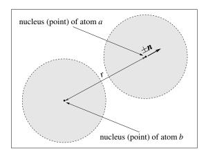
Figure 1: 2D, schematic representation of two atoms, a and b, of a pure substance in the solid state and of the interatomic bond linking a and b – the scale figure is thus approximately  $10^{-1}$ nm. The mass of each atom is mainly concentrated in its nucleus, which is considered as a point. The distance between the nuclei is denoted by r, the unit vector of the direction defined by the nuclei, by  $\pm n$ . The dashed circles provide a simplistic image of the electron clouds.
