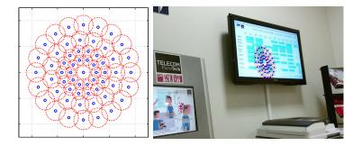
Figure 5: BRISK descriptor sampling pattern from the original implementation (left) and its mapping to the surface through local planar normalization (right).
