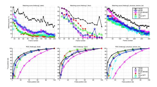
Figure 9: Matching score and receiver operating characteristics demonstrating repeatability and distinctiveness of the compared detectors and descriptors under viewpoint position changes of different kind. Computed on three sequences of *Freiburg* dataset [62], acquired with Kinect. In some images in *desk* sequence and in the whole *floor* sequence VIP turns unable to detect any feature.
