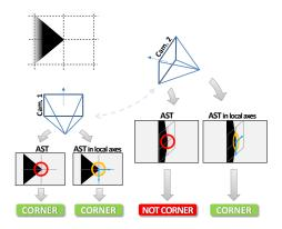
Figure 4: Illustration of application of Accelerated Segment Test (AST) in standard image axis versus local axes derived from the depth map. A corner viewed under a large angle projects itself at a nearly straight contour on the camera plane, so that the corner test in standard image axes fails causing a repeatability loss.
