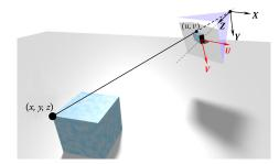
Figure 2: Local camera coordinates (x, y, z) and image plane coordinates (u, v).
