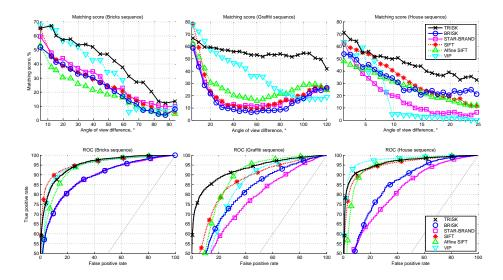
Figure 8: Matching score and receiver operating characteristics demonstrating repeatability and distinctiveness of the compared detectors and descriptors, mainly under out-of-plane rotations (*Bricks* and *Floor* sequences) and scale changes (*House* sequence). Computed on synthetic RGB data. At least 4800 true positive and 4800 false positive matches were selected to plot each ROC curve.
