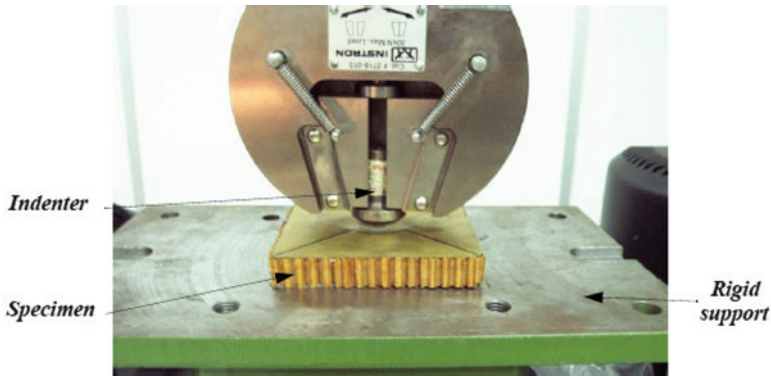
Fig. 29 Description of the indentation tests on sandwich specimens
