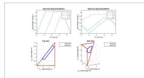
**Figure 23** Comparaison between the abnormal periodic strokes and the experimentally observed stroke. The top figures display the variation of the appendage angles with respect to time. The observed ones reflect the constraint on the angles. The bottom figures show the strokes as closed curves in the triangular prism.
