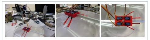
**Figure 25** Set-up of the experiment . The dimensions of the robotics copepod are as follows. The body is a 75 by 43 mm rectangle with four 13 by 23 mm rectangles to fit the motors. The body is 12 mm high with a 10 by 10 hole to fit the rail. Each leg measures 69 mm in length and as a cross section is  $9 \text{ mm}^2$ .
