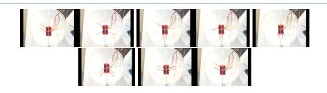
**Figure 28** A sequence of configurations for the copepod during a stroke. The power strokes can be seen in the first 5 snapshots and the return part of the stroke with both legs moving together is displayed in the last three snapshots.
