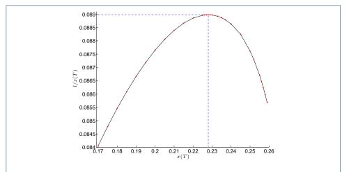
Figure 16 Efficiency curve for the mechanical cost and the corresponding minimizing curve with the best performance is represented in Fig.15. Note that the efficiency of the abnormal curve is  $5.56e^{-2}$  vs of order  $8.89e^{-2}$  for normal strokes.
