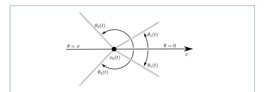
Figure 2 Model of the Copepod micro-robot Sketch of the 2-link symmetric swimmer.
