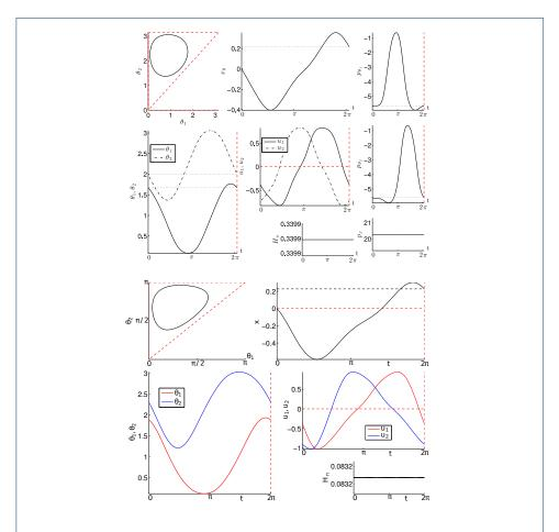
Figure 15 Optimal stroke of the Copepod swimmer for the Euclidean cost (top) and the mechanical energy (bottom), obtained by the transversality conditions of the maximum principle.
