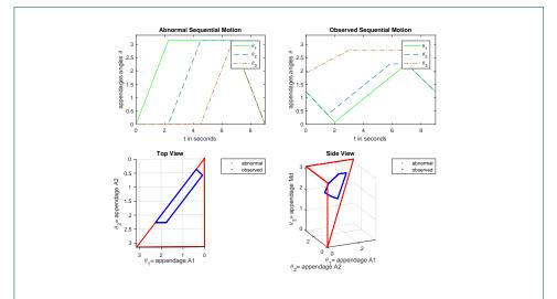
**Figure 22** Comparaison between the abnormal periodic strokes and the experimentally observed stroke. The top figures display the variation of the appendage angles with respect to time. The observed ones reflect the constraint on the angles. The bottom figures show the strokes as closed curves in the triangular prism.
