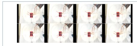
**Figure 26** A sequence of configurations for the copepod during a stroke. The power strokes can be seen in the first 5 snapshots and the return part of the stroke with both legs moving together is displayed in the last three snapshots.
