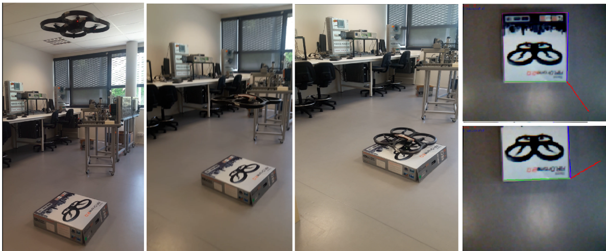
Figure 9. Visual servoing for homing. On the left: the mini-quadcopter hovering above the landing template and performing a controlled landing. On the right: the view seen from the bottom camera of the mini-quadcopter that shows robustness to clutter (when the landing object is partially out of the field of view).
