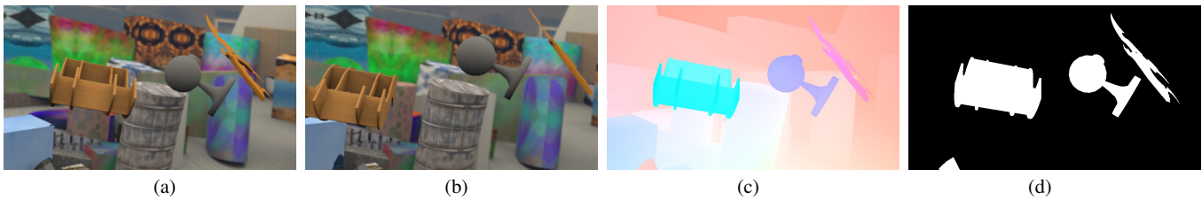
Fig. 2 (a,b) Two example frames from a sequence in the FlyingThings3D dataset [46]. The camera is in motion in this scene, along with four independently moving objects. (c) Ground-truth optical flow of (a), which illustrates motion of both foreground objects and background with respect to the next frame (b). (d) Ground-truth segmentation of moving objects in this scene.
