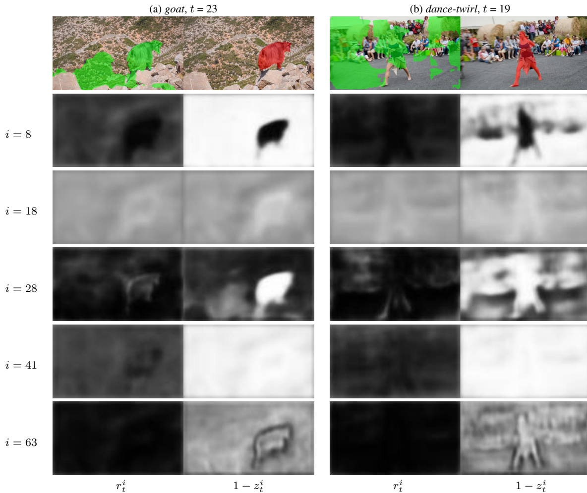
Fig. 11 Visualization of the ConvGRU gate activations for two sequences from the DAVIS validation set. The first row in each example shows the motion stream output and the final segmentation result. The other rows are the reset ( r_t ) and the inverse of the update ( 1 - z_t ) gate activations for the corresponding i th dimension. These activations are shown as grayscale heat maps, where white denotes a high activation.
