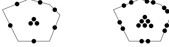
Figure 1: Uncut hexagonal cell. Left: k = 0 ; Right: k = 1 . Each dot symbolizes one degree of freedom (not necessarily a pointwise evaluation).
