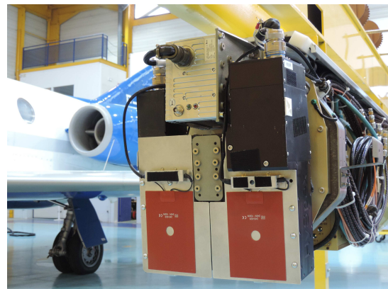
(b): IMU between VNIR and SWIR cameras
