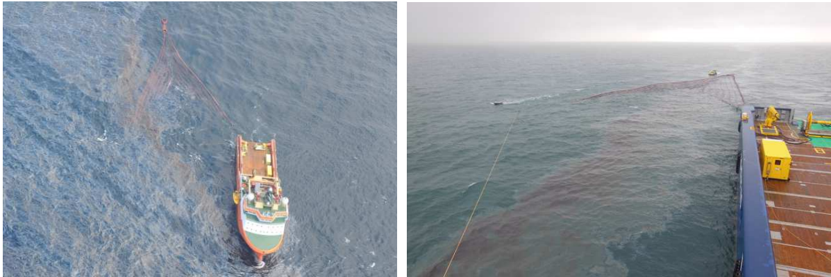
106 Figure 1. MOS Sweeper mechanical recovering system operated by NOFO during trial at sea (photographs 107 provided by NOFO). 108
