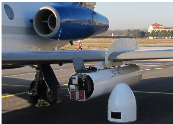
(a): Hyperspectral setting into the nose of left pod
