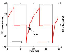
Fig. 5.Voltage and current waveforms in the switches K2 and K1'. The turn-on is done from a positive voltage to a positive current. The turn-off is a passage from a positive current to a negative voltage.
