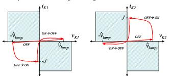
Fig. 6.Identification of the switches to use in the H-bridge. In the left the characteristics for K1 and K2'. In the right the characteristics for K2 and K1'. The four switches are functional SCR thyritors.
