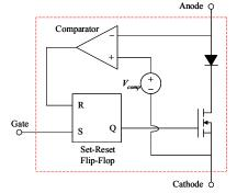
Fig. 7.Functional high frequency SCR thyristor.
