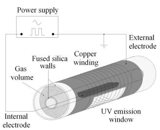
Fig. 1. Experimental set-up of a DBD excilamp.
