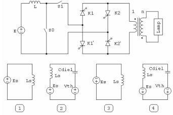
Fig. 9. Boost structure and its four sequences seen from the secondary. The phases 1 and 2 take place when K2 and K1' are ON. The steps 3 and 4 correspond to the conduction of K1 and K2'. Phases 1 and 3 are the positive and negative charge phases.
