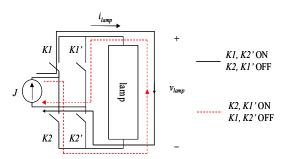
Fig. 4.Ideal H-bridge converter. The continuous or periodic current source J, is sent to the lamp unchanged when K1 and K2' are ON. The current source is inverted when K2 and K1' are ON.
