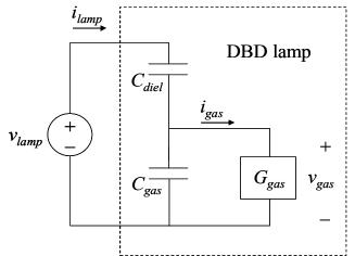
Fig. 2.Electrical model of the DBD lamp.  $C_{gas}$  corresponds to the gas behavior when there is no discharge in the gas.  $C_{diel}$  represents the series equivalent capacitance of the two dielectric walls.
