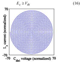
Fig. 12. State plane analysis in the Boost converter. Example of instability for  $E_s$  greater than  $V_{th}$ .
